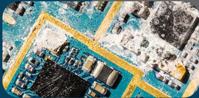
Moisture can cause short circuits, metal corrosion, and component degradation.
